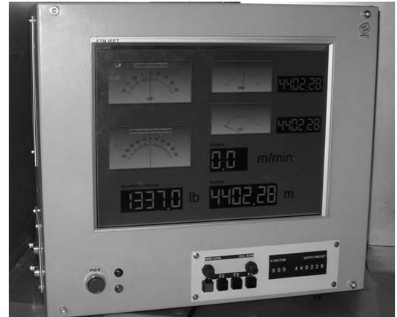
Indoor embedded system for monitoring of critical parameters in borehole measurement (NIS - Naftagas)
