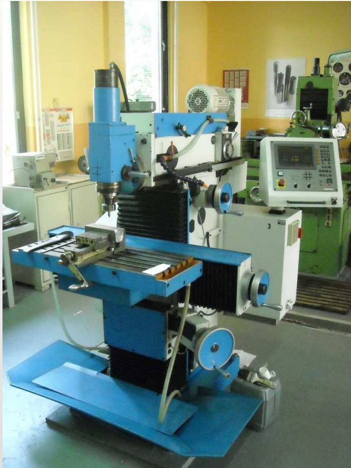
NC milling-boring machine WF 5/800 with Heidenhain control unit
