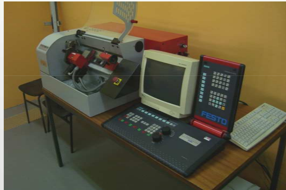
CNC educational turning machine EMCO PC TURN 55, with Sinumeric control unit.
